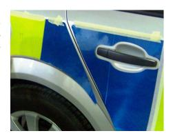
**Step 2.** Remove the liner and squeegee piece into place.
